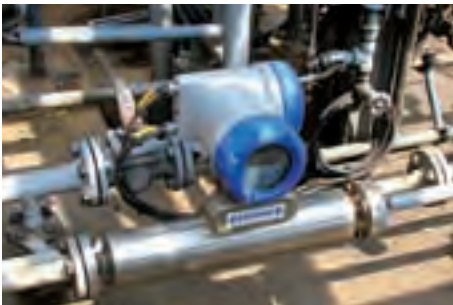
OPTIMASS 7300 with titanium measuring tube in use at AkzoNobel in the Netherlands
