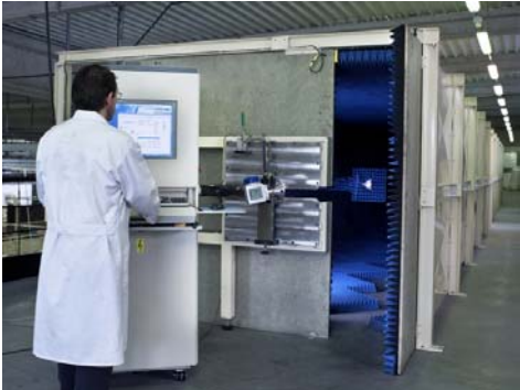
Calibration rig for level measuring instruments
