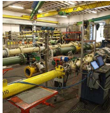
Figure 1: OPTISWIRL 4070 C on the pigsar test rig
