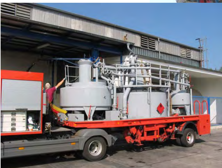
Left: A mobile volumetric calibration system to verify the meters after installation. Normally witnessed by a representative from the local weights and measures authority .
